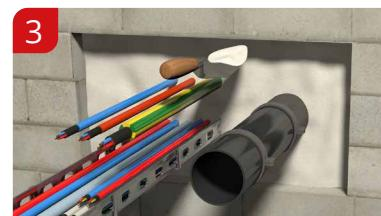
Trowel / Pour the mixture into the wall / floor penetration.
